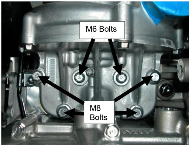
Cover opening on front of engine left when supercharger was removed to prevent debris from entering.
