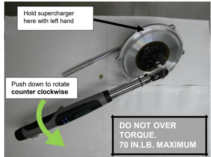
Remove gear holding tool (if used). Spin supercharger impeller to check for smooth operation.
