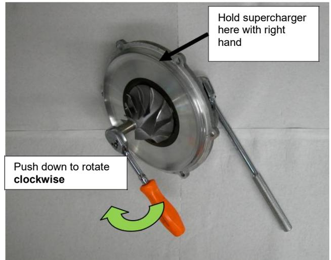
**Note: 2015 & newer models** do not have the 17mm nut on the gear end of drive shaft. Use RIVA part # RY17040-ISH supercharger shaft gear holding tool to hold shaft in place while loosening the 10mm nut. This gear holding tool can also be used on drive shafts that have the 17mm nut, making this process easier than using a 2<sup>nd</sup> ratchet.
