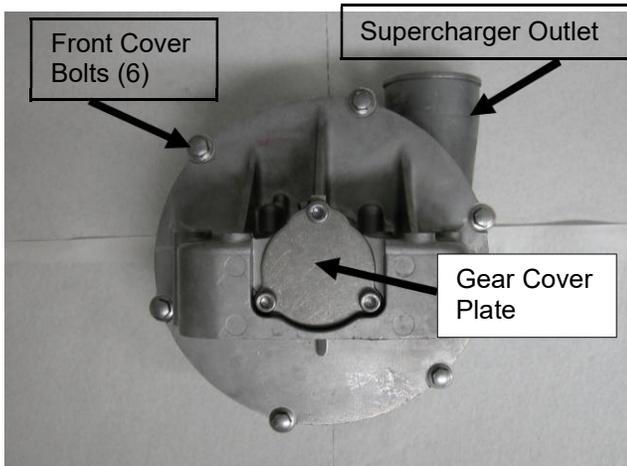
Remove supercharger gear cover plate and gasket. Remove supercharger cover. **Note:** It may be necessary to lightly tap outlet on supercharger cover to free it from supercharger. **Take care not to damage supercharger cover.**
