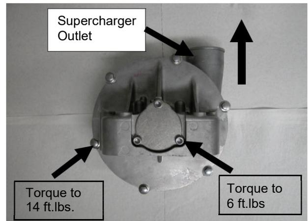
Secure supercharger cover using stock bolts. **NOTE: Apply blue Loctite to bolts. Torque bolts to 14 ft•lb.** Clean excess sealant from edge of supercharger
