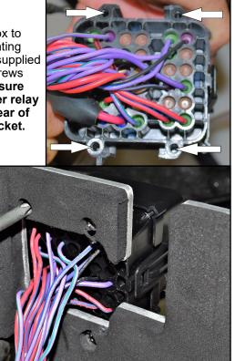
Secure regulator/rectifier to electrical mounting bracket using supplied M6x20 SHCS (2) and M6 flat washers (2) so that connectors face left side of craft. **NOTE: Apply blue Loctite to threads. Do not overtighten.**
