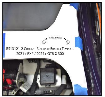
Drill holes using 1/4" drill bit. Do not countersink holes.
