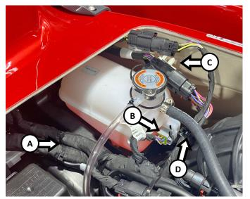
Remove diagnostic connector (B) from engine coolant tank.
