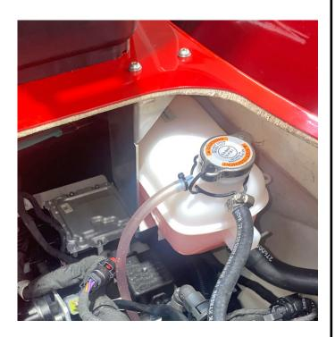
Secure to bracket at front using supplied zip tie and at rear using supplied push pin dart. **NOTE: Be sure zip tie is locked into grooves on bracket.**
