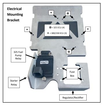
ALL 325hp Models: Install fuel pump relay onto supplied electrical mounting bracket and secure with supplied hardware: M6x25 SHCS (2), M6 wave washers (2), M4x25 SHCS (1) & M4 wave washer (1). NOTE: Apply blue Loctite to threads. Do not overtighten.
