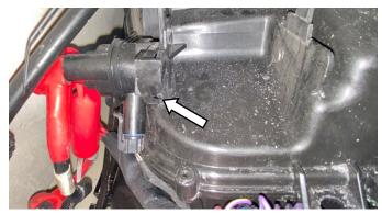
Disconnect electrical connector on starter relay and disconnect electrical connectors (2) from regulator/ rectifier.
