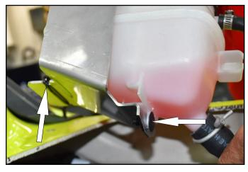
Secure electrical wiring and coolant hose to fuel rail using supplied zip ties.
