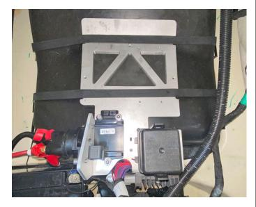
Mount ECU to electrical mounting bracket and secure using supplied hardware.
