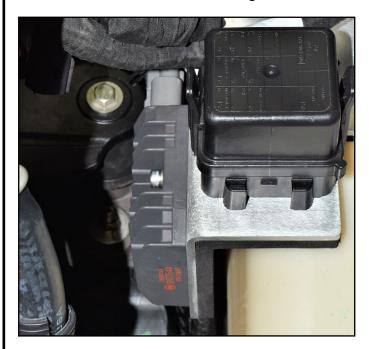
Secure starter relay to electrical mounting bracket using supplied M6x12 SHCS (2) and M6 flat washers (2).**NOTE: Apply blue Loctite to threads. Do not overtighten.**
