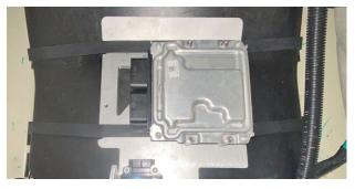
**300/230hp Models:** M6x16 SHCS (3), M6 wave washers (3) & black nylon spacers (3). **NOTE:** Place black nylon spacers between ECU and mounting bracket. Electrical connectors will face rear of craft.
