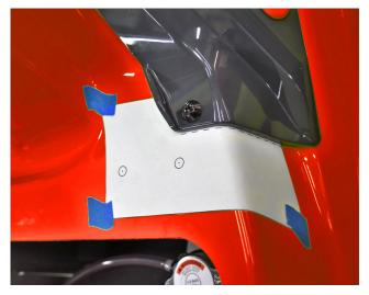
Drill holes using 1/4" drill bit. Holes must be countersunk so that screw heads don't interfere with seat gasket.
