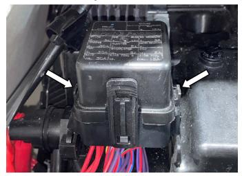
Remove starter relay by prying locking tab outward and then lifting relay upward.
