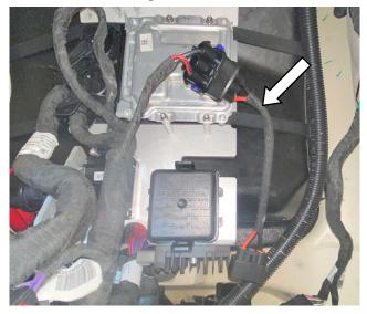
Secure wiring with supplied zip ties.
