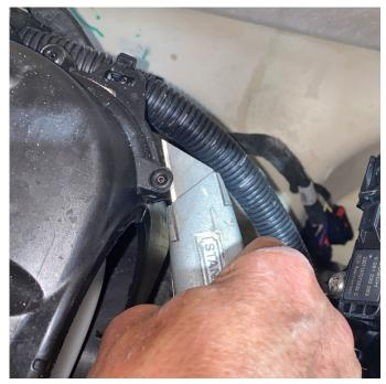
Carefully rotate airbox on top of fuel tank to access rivets at sides.
