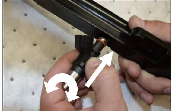
Install injectors so electrical connectors face up when fuel rail is reinstalled. **NOTE: Install so that electrical connector is closest to fuel supply rail.**
