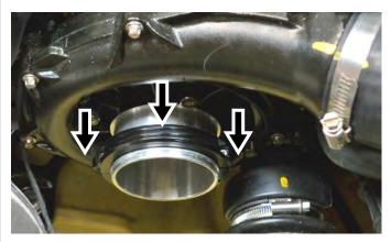
Install supplied tapered adapter onto threaded clamping ring. **NOTE: Do not over tighten.**
