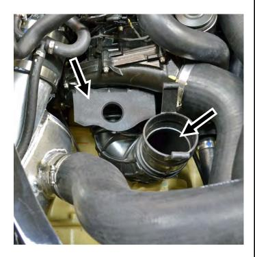
Remove supercharger inlet hose (1 clamp) and discard.
