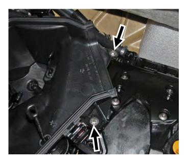
Squeeze outlet hose inside air intake silencer. Remove air intake silencer by lifting up and discard.
