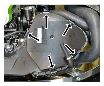
Remove air intake silencer baffle (pull up) and discard.
