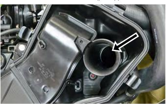
Remove rubber latches (3) securing air intake tube. Remove air intake tube and discard.
