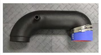
Spray glass cleaner generously onto outside of tapered plastic flange and inside of coupler on Power Filter Tube.
