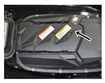
Remove bolts securing engine coolant tank (3) and air inlet (3) to deck extension lid.
