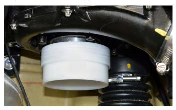
Install supplied coupler onto supplied Power Filter Tube. Loosely install clamps onto coupler (do not tighten).
