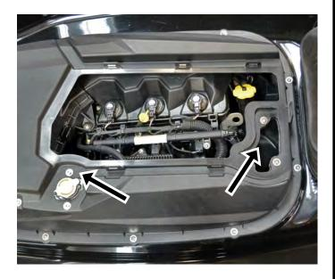
Remove bolts (12) securing deck extension lid to hull.
