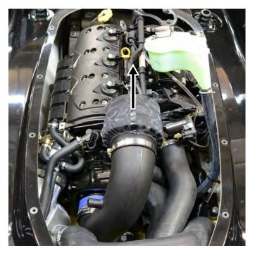
Rotate Power Filter tube so that Power Filter is centered with fuel injectors. Tighten clamps securing coupler to tapered adapter and Power Filter Tube. **NOTE: Do not overtighten clamps.**
