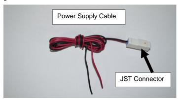
Plug in female JST connector on power supply cable to male JST connector on gauge adaptor cable. **Do not connect power supply cable to communication connector on gauge.** This will damage the gauge.
