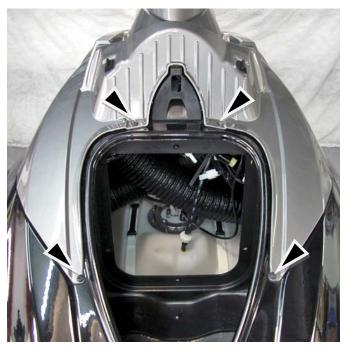
Remove bolts (2) securing reverse lever handle. Remove handle and set aside.
