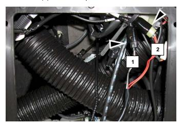
**TIP:** Trace wires from the end of steering shaft (inside hull) to their connection points.
