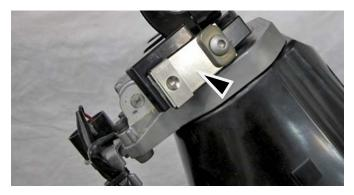
Install supplied Bar Mount System onto head of steering stem. NOTE: Apply red Loctite to bolts. Torque evenly to 14 ft•lb / 19 N•m.
