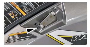
Remove bolts & nuts (1 set per side) securing lower rear sides of hood cowling to hull.
