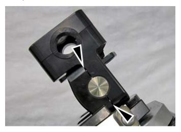
Transfer steering arm ball joint and lock nut from stock steering arm to supplied billet steering arm.
