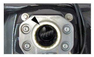
Remove bolts (4) securing instrument gauge to hood cowling.
