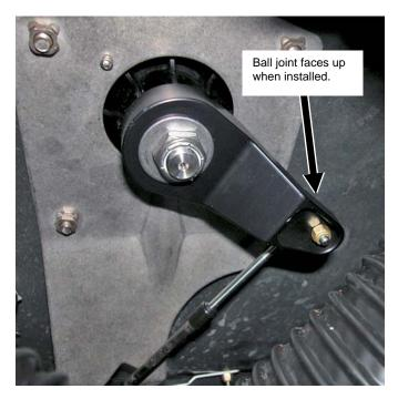
Install supplied washer and secure with supplied nut. **NOTE:** Tighten nut until you are no longer able to turn upper portion of steering freely by hand.
