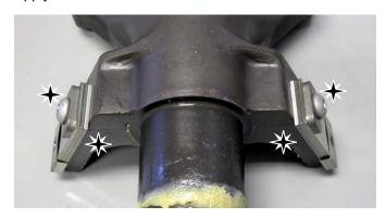
Remove OTS bolts and board springs. **NOTE: If bolts** do not loosen easily apply more heat. Take care not to burn yourself. *Components will be very hot!*
