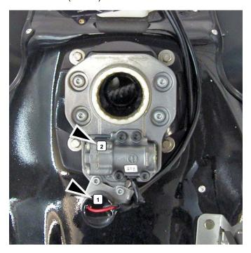
At base of steering column remove bolts (4) securing column to hull.
