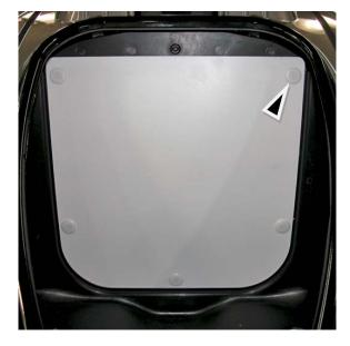
TIP: Push center of rivets in to release.
