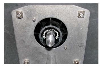
Install small billet collar onto end of steering shaft and into housing assembly.
