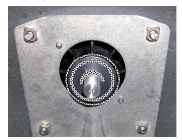
Install supplied billet steering arm onto end of steering shaft. **NOTE:** Arm is machined to fit over billet collar.
