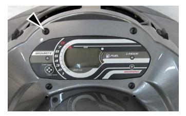
Remove bolts & nuts (4) securing front of hood cowling to front of craft.
