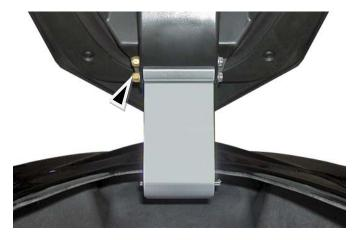
Inside front storage compartment remove service lid (5 rivets).
