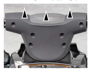
Inspect steering column for plastic collar (bearing). If it is not present remove from steering shaft and install into column.
