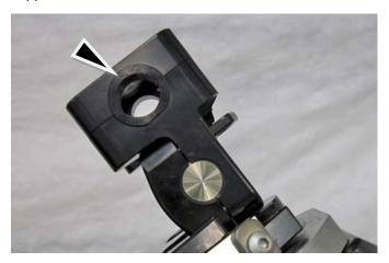
NOTE: Thoroughly clean bars, billet spacers and handlebar clamping surfaces with a non-residual cleaner. Apply red Loctite to handlebar clamp bolts. Torque bolts evenly to 14 ft•lb / 19 N•m.
