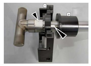
Apply waterproof grease to outside of upper collar <sup>2</sup>. Insert steering assembly into steering column. **NOTE: Billet steering stop faces rear of craft.**
