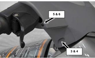
Remove throttle cable from throttle trigger.
