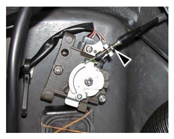
At top edge of service opening disconnect electrical connectors (2) for start/stop switch.
