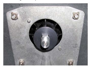
Coat billet collar and end of steering shaft with waterproof grease.
