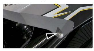
Inside front of hull remove bolts (2 per side) securing hood cowling to hull.
