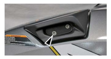
Remove bolts (2) securing hood cowling to reverse lever assembly.
