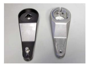
**NOTE:** We have provided three installation options. The center is equal to stock. Inside option will move steering nozzle faster. Outside will move steering nozzle slower. Always check steering cable travel to ensure steering locks on billet steering stop and not the actual cable.
