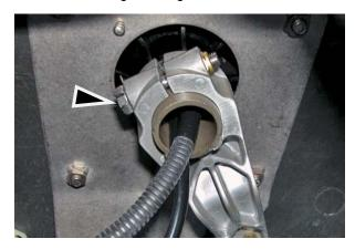
Pry locking tabs away from head of bolt. Remove bolt completely.
