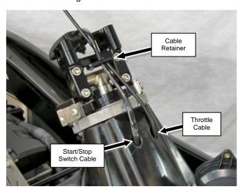
Pull throttle cable and start/stop switch wires through bottom of steering column and reconnect.
