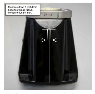
Drill a pilot hole at 3/4" out from each side of center line 1" down from bottom of small radius. **NOTE: Do not apply heavy pressure when drilling.**
