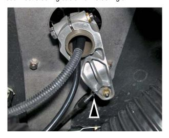
Locate bolt securing steering arm to main shaft.
