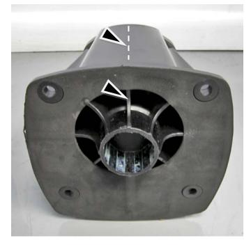
Using a straight edge draw a reference line along reinforcement rib on front of steering column.
