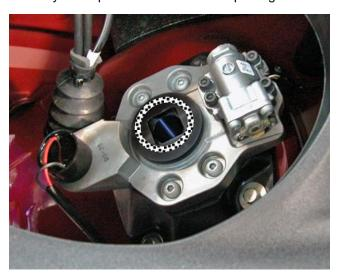
Install small plastic collar onto supplied small billet collar. Coat plastic collar with waterproof grease.
