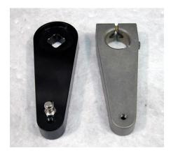
**NOTE:** We have provided three installation options. The center is equal to stock. Inside option will move steering nozzle faster. Outside will move steering nozzle slower. Always check steering cable travel to ensure steering locks on billet steering stop and not the actual cable.
