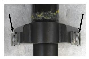
Remove OTS bolts and board springs. **NOTE:** If bolts do not loosen easily apply more heat. Take care not to burn yourself. *Components will be very hot!*
