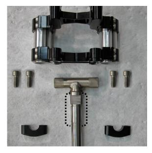
Apply generous amount of waterproof grease around top of stainless steel steering shaft (see detail area above).
