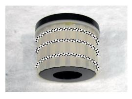
Install large billet collar into top of steering housing assembly. Coat plastic collar with waterproof grease.
