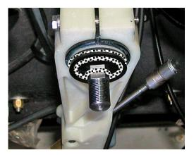
Transfer steering ball joint and lock nut from stock steering arm to supplied billet steering arm.
