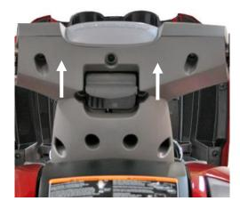
Remove plastic collars (1 large/1 small) from steering shaft.
