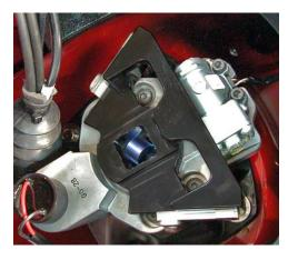
Secure supplied billet steering shaft to supplied steering riser. Thoroughly clean clamping components where they join using a non-residual cleaner. NOTE: Apply red Loctite to clamp bolts. Torque bolts evenly to 14.8 ft-lb / 20 N-m.
