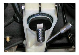
Coat billet collar and end of steering shaft with waterproof grease.
