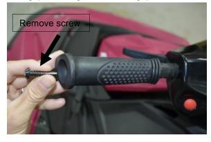
Align RIVA bar extension with notch in OE handlebar and install. Secure in place using OE grip retaining screw.
