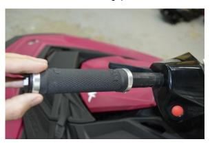
**Note:** If using ODI locking grips, tighten screws on locking rings at ends of grip.
