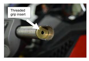
Install RIVA handlebar extension on end of OE handlebar.
