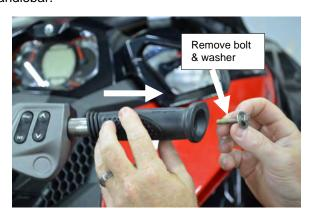
Ensure threaded grip insert is properly seated on the OE handlebar.
