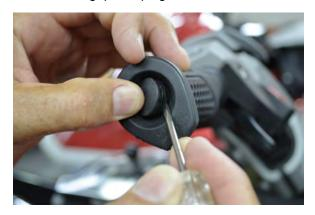
Remove grip retaining bolt & washer. Slide grip off of handlebar.
