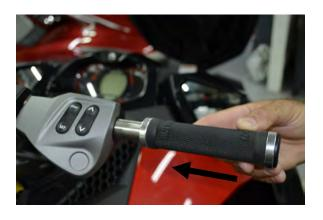
**Note:** If using ODI locking grips, tighten screws on locking rings at ends of grip.
