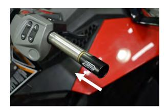
Secure RIVA bar extension using OE grip bolt & washer. Note: Apply blue Loctite to bolt. Torque to 7 Nm (62 inch lbs.)
