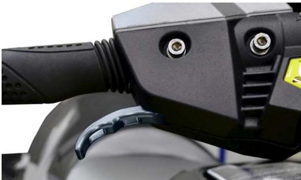
**NOTE: Apply blue Loctite to threads. Torque bolts to 18 lbf•in / 2 N•m.**
