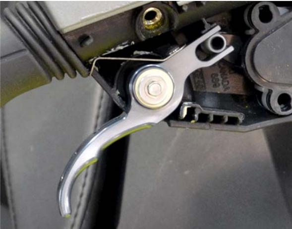
**NOTE: DO NOT OVER TIGHTEN BOLT. Apply blue Loctite to threads. Torque bolt to 6 lbf•in / 0.7 N•m.**
