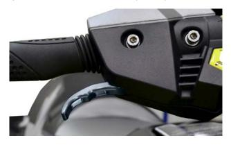
NOTE: Apply blue Loctite to threads. Torque bolts to 18 lbf•in / 2 N•m.
