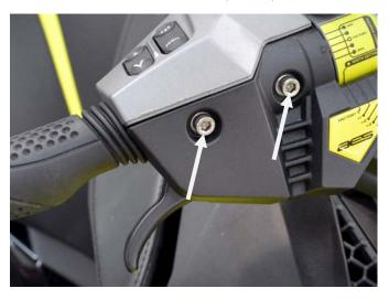
Remove bolt and washer securing stock lever.
