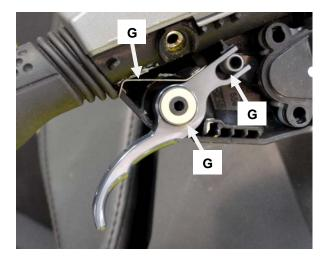
Secure with stock bolt and washer.
