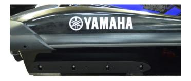
Install left side RIVA sponson blade onto billet backing plate using 5 of the supplied button head allen screws and wave lock washers.
