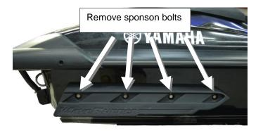
Install right side billet backing plate using 4 supplied allen head bolts & flat washers. **Note:** We suggest first starting in the middle bolt position on the backing plate. **Use blue Loc-Tite.** *Do not over tighten bolts.*
