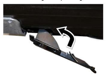
Remove intake grate. Apply generous amount of 'below waterline' silicone sealant to front of transom plate.
