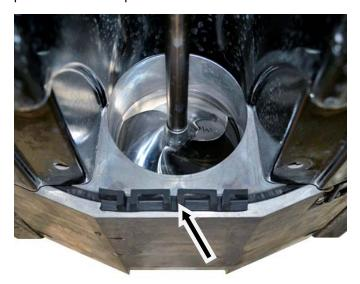
**TIP:** Loosen front bolts (2) as much as possible, but do not remove completely.
