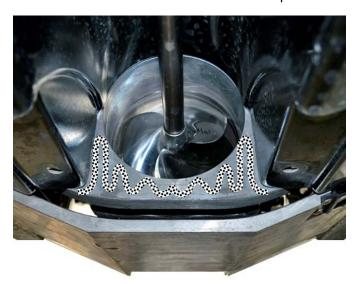
Apply generous amount of 'below waterline' silicone sealant to edges/sides of intake grate and front of intake grate.
