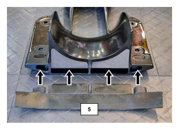
Before installing intake grate permanently test fit to ensure intake grate seats properly in hull. Variances in materials (hull, transom plate, pump seal kit) may require the Pump Seal Kit be relieved to allow intake grate to be installed properly.
