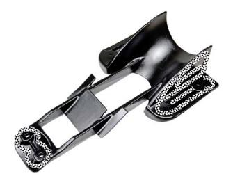
Install intake grate and secure with stock bolts. NOTE: Apply blue Loctite to bolts. Torque to 12.5 lbf•in / 17 N•m.
