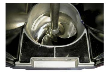
Insert the two narrow pieces of Pump Seal Kit into rear opening of RIVA SS Intake Grate.
