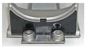
Test fit intake grate to ensure it seats properly in hull. Variances in materials (hull, transom plate, pump seal kit) may require the Pump Seal Kit be relieved to allow intake grate to be installed properly.
