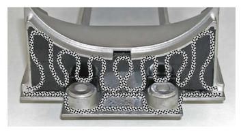
Apply generous amount to edges/sides of intake grate and front of intake grate.
