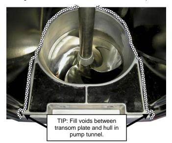
Apply a generous amount of 'below waterline' silicone sealant to all exposed surfaces of pump seal kit inserts in intake grate.
