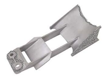
Install intake grate and secure with stock bolts. **NOTE: Apply blue Loc-tite to bolts. Torque to 29 lbf•in / 40 N•m.**
