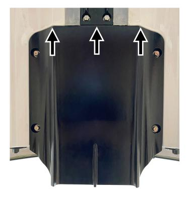
Install supplied RIVA ride plate using OEM bolts making sure front edge of ride plate is against hull and pump inlet shoe evenly.
