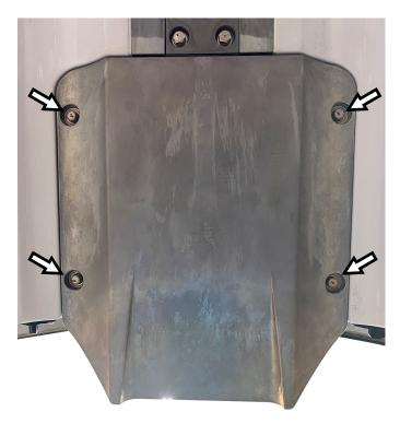
Remove OEM ride plate bolts (4). If necessary, use a heat gun to apply heat to *bolt heads only*!
