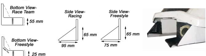
NOTE- RIVA SuperJet Rear Hull Extensions are supplied with oversize length to allow for "trimmable" ride adjustment after installation.
