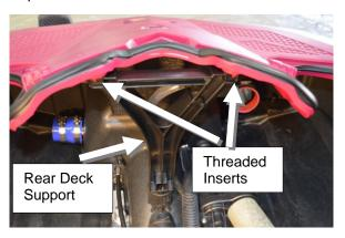
Step 23: Reinstall top deck to lower deck (refer to step 11) Guide steering cable through cable access hole on top deck. Use care to ensure the rubber deck seals are properly sealing. Line up screw holes between the top & lower deck.
