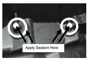
Step 18: Position supplied threaded hull inserts over the mounting holes on the inside of the hull. **Note:** Three of the hull inserts are identical. The one dissimilar insert is to be installed on the mounting hole near the boarding step.
