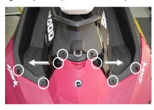
Step 9: Remove the ten (10) circled Torx screws & nuts on the sides of the hull. (see illustration below)
