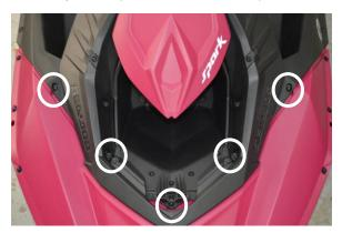
Step 8: Remove the eight (8) circled self tapping screws at the rear of the top deck. Remove rear trim pieces by sliding out of position. (see illustration below)
