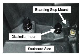
Step 19: Apply a generous bead of Permatex "The Right Stuff" or equivalent around the mounting areas on the trim tab. (see illustration below)
