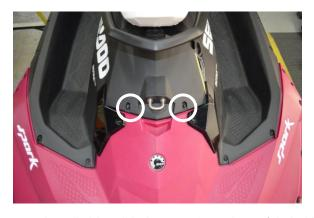
Step 26: Install side rail bolts, nuts & washers. (circled in illustration below) Torque to 3.5 N.m / 31 inch lbs.
