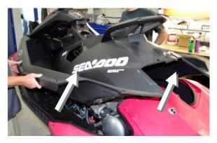
Step 12: Remove the Torx screws on rear deck panel and remove panel. (see illustration below)
