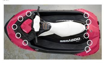
Step 28: Reinstall self taping screws (3) at gas fill cap. Torque to 4.5 N.m / 40 inch lbs. (refer to step 10)
