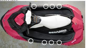
Step 27: Reinstall rear trim pieces (refer to step 8) & reinstall self tapping screws at front & back of hull. (circled in illustration below) Torque to 5.5 N.m / 49 inch lbs.
