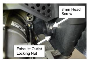
Step 14: Loosen hose clamp on water box outlet hose and remove exhaust resonator box from hull.
