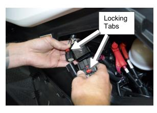
Step 4: Remove left side knee pad by pulling on right side of panel.
