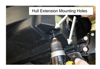
Step 16: After all four mounting holes have been drilled from the underside, **SLOWLY** drill the four mounting holes from the top side of the hull using a "B" size drill bit. **Note:** Use your drill on the low speed setting & drill as straight as possible.
