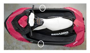
Step 25: Install rear support screws (circled in illustration below) Torque to 5.5 N.m / 49 inch lbs.
