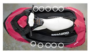
Step 10: Remove three (3) self tapping screws located at the fuel fill cap.
