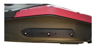
Install left side RIVA sponson blade onto billet backing plate using 4 of the supplied shorter bolts & washers. **Note:** We suggest first starting in the middle area bolt position on the sponson blades. **Use blue Loc-tite. Do not over tighten bolts.**
