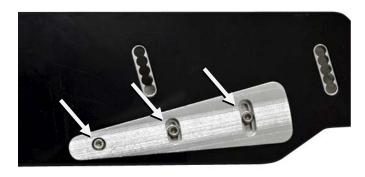
After finding your favorite position remove bolts one at a time, apply blue Loctite to threads and replace. **Torque** bolts to 3.5 ft•lb / 44 in•lb / 5 N•m.
