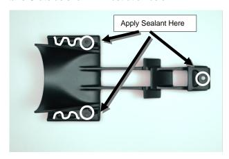
Install Top Loader Intake Grate in position on underside of hull. Loosely install the 3 front intake grate bolts, washers & retaining nuts. (Or, bolts & washers only if using the RIVA Intake Grate Backing Plate Kit (part# RS21130-BPK-RI) **Tip:** Have someone hold the retaining nuts in place when installing the intake grate bolts.
