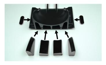
Before installing intake grate permanently, test fit to ensure intake grate seats properly in hull. Variances in materials (hull, transom plate, pump seal kit) may require the Pump Seal Kit be relieved to allow intake grate to be installed properly.
