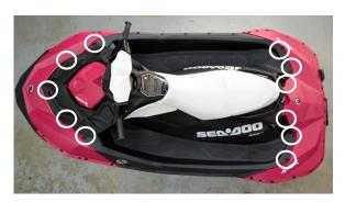
Step 25: Reinstall self taping screws (3) at gas fill cap. Torque to 4.5 N.m / 40 inch lbs. (refer to step 10)
