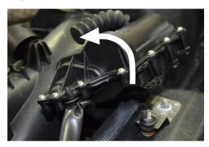
Step 14: Using a long socket extension, remove the two rear inlet grate self tapping screws (8mm head) located just under jet pump. (circled in illustration below)
