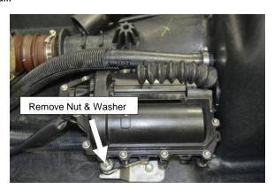
Carefully rotate IBR actuator counter clockwise.
