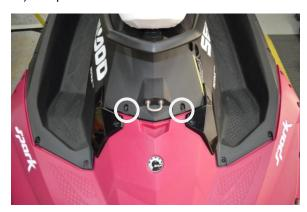
Step 23: Install side rail bolts, nuts & washers. (circled in illustration below) Torque to 3.5 N.m / 31 inch lbs.
