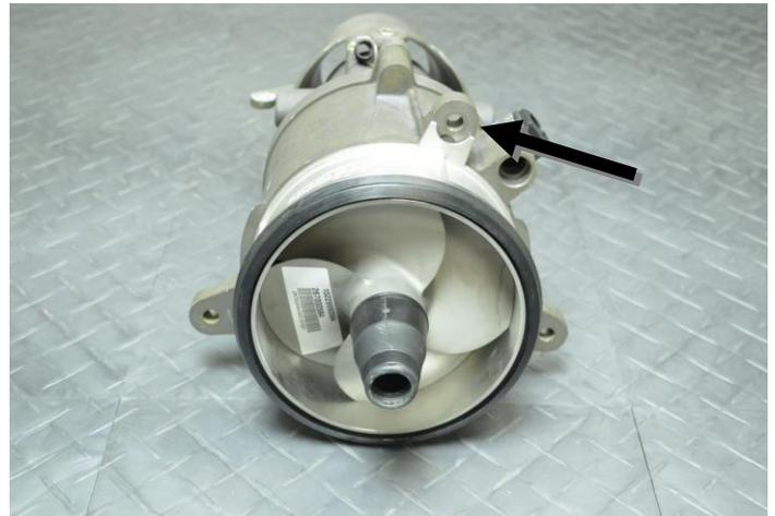
**IMPORTANT:** Note position of radiused tab on Stainless Steel Wear Ring.
