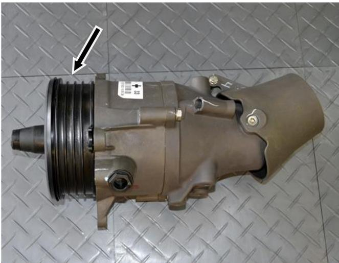
Transfer rubber seal from stock plastic wear ring to supplied Stainless Steel Wear Ring.
