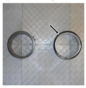
Install Stainless Steel Wear Ring onto pump.
