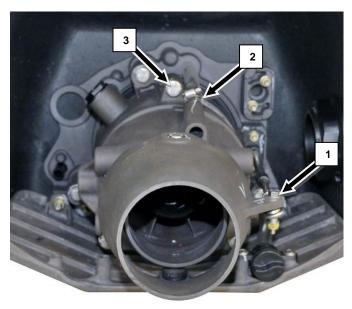
Remove plastic siphon bilge fitting<sup>2</sup> from top of reduction nozzle.
