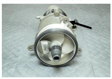
IMPORTANT: Note position of radiused tab on Stainless Steel Wear Ring.
