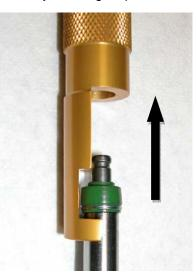
**TIP:** While lifting with one hand use other to apply slight downward pressure on opposite end of tool to prevent
