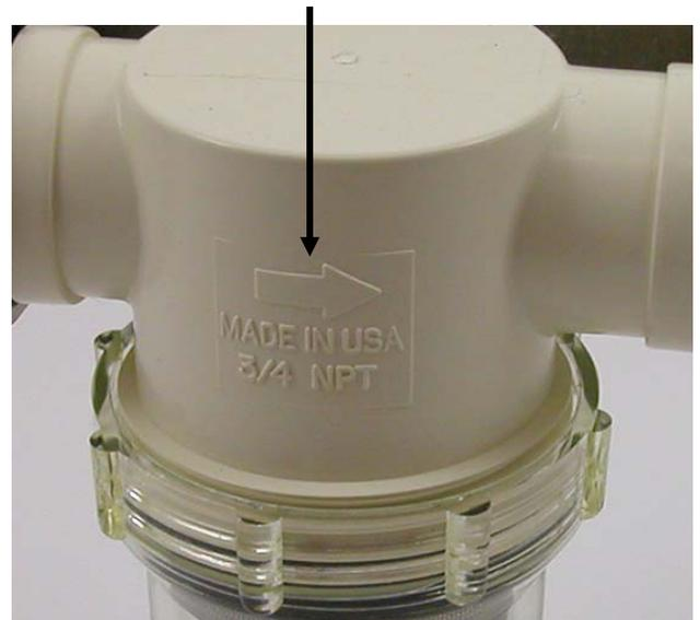
Apply pipe thread sealant to threads on barbed fittings. Align filter in bracket so that barbed fittings can be installed through large openings and into filter.
