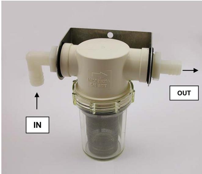
Tighten 90-degree fitting until it faces downward when snug. Install straight fitting until it is snug. **NOTE: Do not over tighten fittings. If fittings are removed reapply pipe thread sealant before replacing.**
