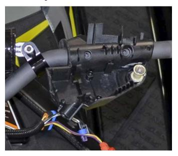
Replace control buttons, lever switches and reconnect electrical connectors.
