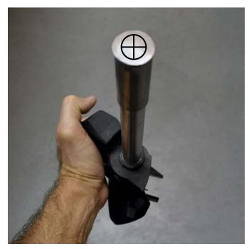
While holding housing in one hand strike large end of tool with a heavy steel hammer. Repeat until steel pipe is driven out of housing completely.
