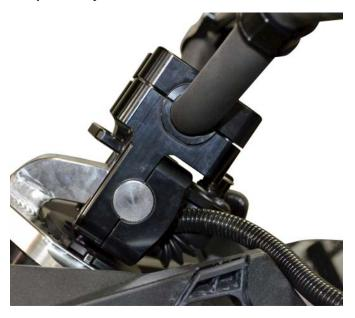
Install housings onto handlebars.
