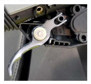
NOTE: DO NOT OVER TIGHTEN BOLT. Apply blue Loctite to threads. Torque bolt to 6 lbf•in / 0.7 N•m.
