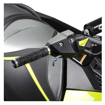
NOTE: Apply blue Loctite to threads. Torque bolts to 18 lbf•in / 2 N•m.
