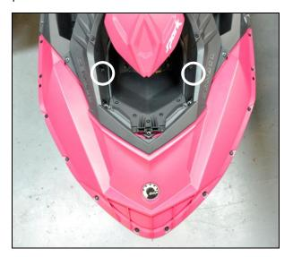
The top main deck needs to be removed in order to access the M6 elastic nuts. When these bolts are removed, replace plastic washers with upgraded washers. Reinstall & torque bolts to 4.5 Nm +/- 0.5 Nm. (40 inch lbs. +/- 4 inch lbs.)
