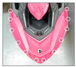
Discard plastic washers. Reinstall Torx screws and upgraded washers in place of plastic washers. Torque to 5.5 Nm +/- 0.5 Nm. (49 inch lbs. +/- 4 inch lbs.)
