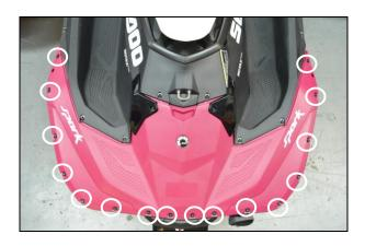
Discard plastic washers. Reinstall Torx screws and upgraded washers in place of plastic washers. Torque to 5.5 Nm +/- 0.5 Nm. (49 inch lbs. +/- 4 inch lbs.)
