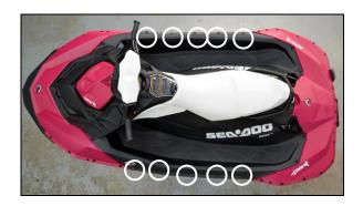
Discard plastic washers. Reinstall Torx bolts, upgraded washers in place of plastic washers, and nuts. Torque to 3.5 Nm +/- 0.5 Nm. (31 inch lbs. +/- 4 inch lbs.)
