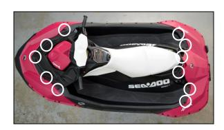
Discard plastic washers. Reinstall self tapping Torx screws & upgraded washers in place of plastic washers. Torque to 5.5 Nm +/- 0.5 Nm. (49 inch lbs. +/- 4 inch lbs.)
