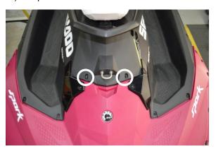
39. Install side rail bolts, nuts & washers. (circled in illustration below) Torque to 3.5 N.m / 31 inch lbs.
