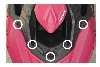
8. Remove the eight (8) circled self tapping screws at the rear of the top deck. Remove rear trim pieces by sliding out of position. (see illustration below)
