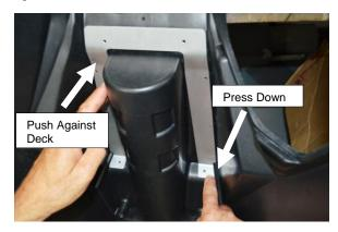
14. While holding bracket in position against the hull, drill the bottom right side bolt hole using a 5/32" size drill bit.
