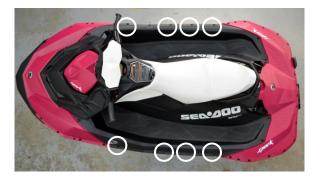
40. Reinstall rear trim pieces (refer to step 8) & reinstall self tapping screws at front & back of top deck. (circled in illustration) Torque to 5.5 N.m / 49 inch lbs.
