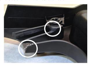
33. Position the supplied access panel bracket on the inside of the top deck. Secure in place using the 6 supplied M4 flat head bolts, washers & nuts. **Do not over tighten.**
