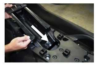
47. Secure access panel in place using the 2 supplied bolts. Tighten by hand. **Do not over tighten bolts.**
