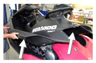
12. **2up Models:** Remove bolts (4) securing rear grab handle to top deck & remove handle.
