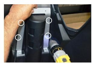
17. Using a #2 pencil, mark the two top mounting bracket holes.
