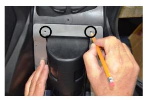
Remove bracket & bolts. Drill the marked top holes using a 13/64" size drill bit.
