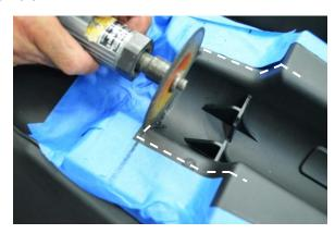
26. Cut just above the pencil line as shown in the illustration below. **Note:** Take your time with this cut. You want to "sneak up" on the left & right corners.
