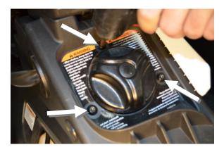
11. With assistance, remove top deck by lifting straight up from lower deck. Guide steering cable through cable access hole in top deck.
