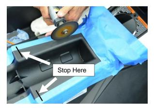
24. Cut the front section of the fire extinguisher area. Cut on the INSIDE of the perforated pencil line.
