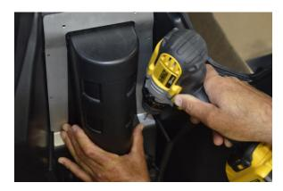
Install one supplied M4 flat head bolt to hold the bracket in place.
