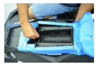
29. Using a hand file, file down the left & right rear corners of the cut out. (see illustration below)
