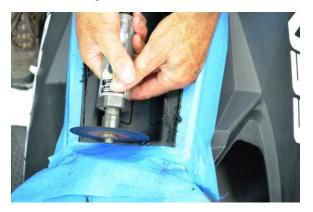
25. Cut the rear of the fire extinguisher section as shown in the illustration below. **Cut on the INSIDE** of the **perforated pencil line**. You want to "sneak up" on the corners.
