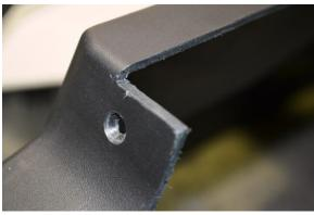
Using a hand file and/or a sander, make adjustments and clean the edges of the cut out. Square the corners using a hand file & ensure the access panel fits properly.
