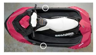
38. Install rear support screws (circled in illustration below) Torque to 5.5 N.m / 49 inch lbs.
