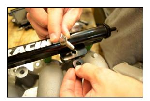
Apply blue Loctite to threads of each bolt & torque to 9.6 ft. lbs. (13 Nm)
