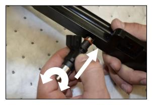
Install injectors so electrical connectors face up when fuel rail is reinstalled. **NOTE: Install so that electrical connector is closest to fuel supply rail.**
