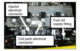
Disconnect electrical connectors (4) from fuel injectors.
