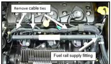
Place an absorbent shop rag under fuel rail supply fitting at front of intake manifold. Carefully disconnect fitting by releasing (slightly lifting) locks using Sea Doo tool (part#529036037) or similar. (see illustration) **Note: Fuel line is under pressure.**
