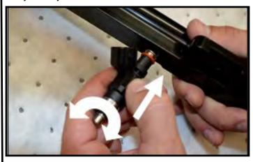
Apply a thin coat of engine oil to the bottom o-ring on injectors.
