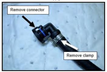
Reinstall fuel supply line onto barbed fitting on front of fuel rail. Secure line to fitting using supplied Oetiker clamp.
