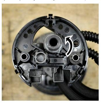
Carefully remove fuel supply hose from fitting at underside of fuel pump module. **NOTE:** You will need to slice the hose at the fitting. Take care not to damage fitting.
