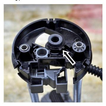
Install supplied fuel hose between fuel pump fitting and underside of fuel pump module. Secure using supplied Oetikers. **NOTE: Ensure pointed tab on fuel pump fitting is still secured between posts.**
