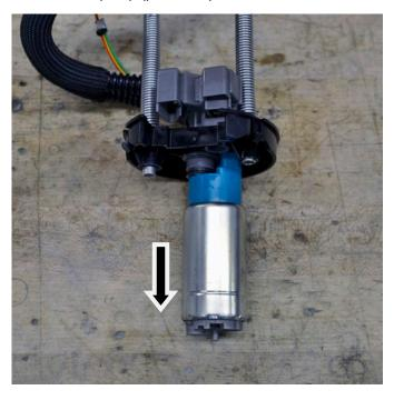
Disconnect electrical wires and set aside. Discard pump.
