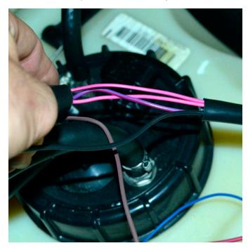
Splice (cut) 'B' wire and reconnect using supplied heat shrink butt connector including red wire from relay.
