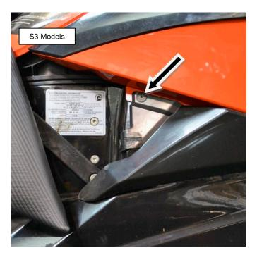
Using supplied hardware secure relay to inside of hull so that wires hang downward.
