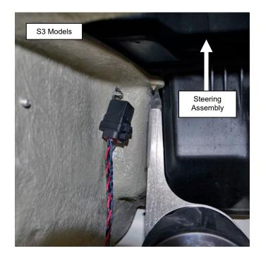
Disconnect fuel pump module electrical connector (if connected).
