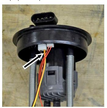
Remove lower section of fuel pump module by *carefully* prying open tabs (3) securing lower section to upper section.
