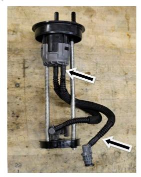
Transfer rubber grommet from inside of stock fuel pump fitting to inside of supplied billet fuel pump fitting.
