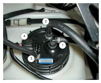
Cover fuel supply hose connector with a shop rag to prevent fuel spill.
