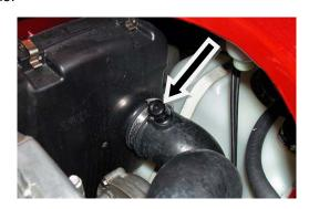
Install supplied breather hose with filter onto engine breather box. Secure using stock spring clamp.
