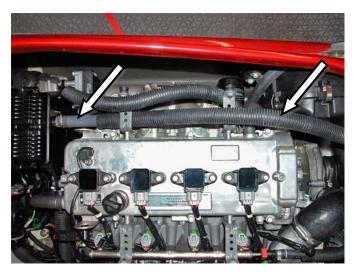
**NOTE:** If retaining stock air intake system leave barbed fitting in hose between air box and supercharger or throttle body.
