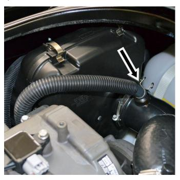
**NOTE:** If retaining stock air intake system leave barbed fitting in hose between air box and supercharger or throttle body.
