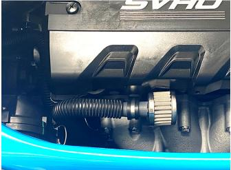
Wide Engine Covers: Secure to underside of bracket using reusable OEM zip tie. NOTE: Ensure end of protective plastic sheathing is pulled up against spring clamp.
