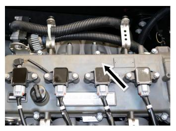
Replace plastic engine cover. **NOTE: Apply blue Loctite to screws. Do not over tighten.**
