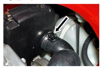
Install supplied filter into open end of engine breather hose. Secure using stock spring clamp.
