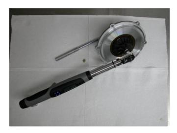
NOTE: The following step requires a 24~240 in•lb electronic torque wrench. A 1/4" drive is recommended, but a 3/8" drive will work. If an IN•LB torque wrench is not available DO NOT PROCEED until you locate one. DO NOT USE A CLICK-TYPE OR FT•LB TORQUE WRENCH.
