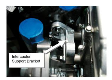
Remove the M8 bolts (4), and M6 bolts (2) from supercharger unit. Remove supercharger unit from engine.
