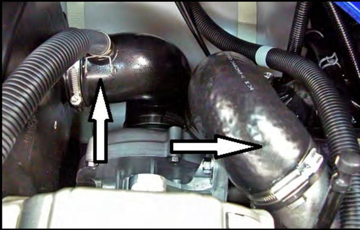
Cover supercharger air outlet and intercooler air inlet with masking tape to prevent debris from entering.
