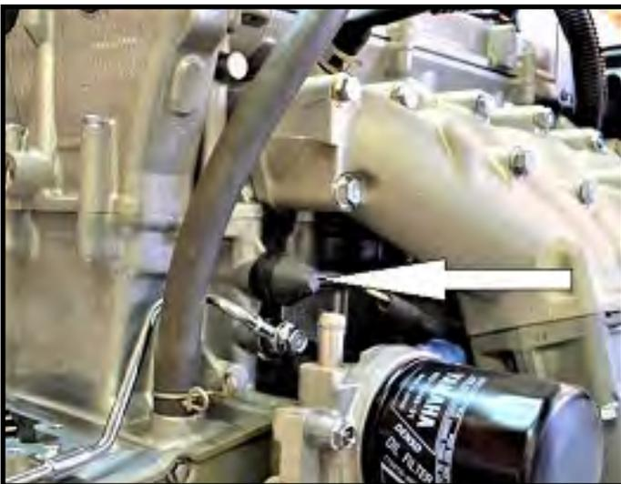
Remove screw securing oil pressure to wire harness connector. (Figure 24) Remove oil pressure switch.
