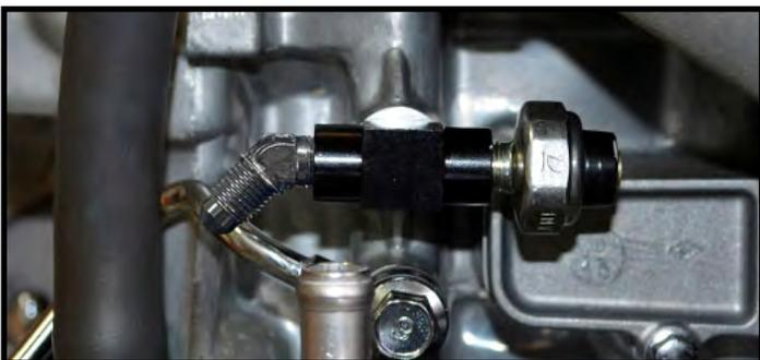
Reconnect oil pressure switch electrical wire and replace rubber boot.
