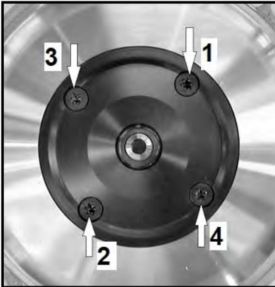
Remove screws (4) holding thrust plate. (Figure 11) Remove thrust plate and step collar.
