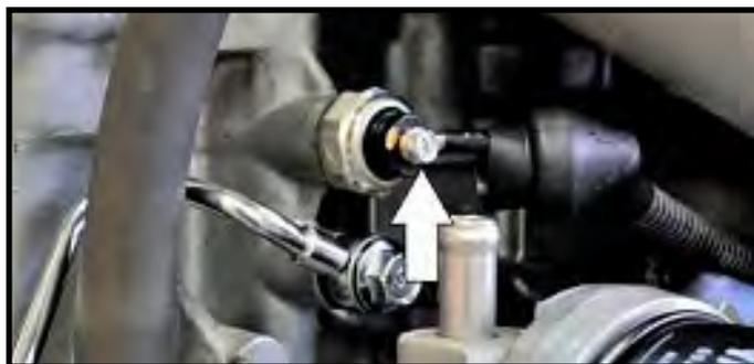
Install supplied billet 'T' fitting into engine crankcase (figure 25). Tighten until side of fitting with machined dot faces rear of engine/craft. **NOTE: Apply pipe thread sealant to male pipe threads. Do not over tighten billet 'T' fitting.**
