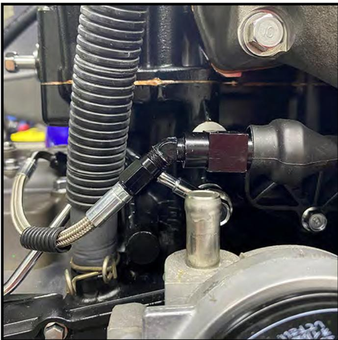
Replace oil cooler bypass hose and secure with stock clamp.
