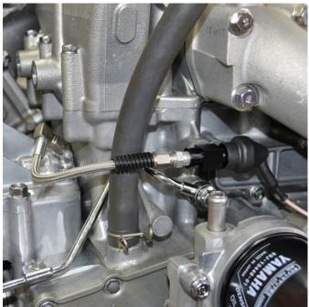
NOTE: Secure JIC fitting in billet 'T' fitting before applying final torque to braided line fitting.
