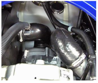
Cover supercharger air outlet and intercooler air inlet with masking tape to prevent debris from entering.
