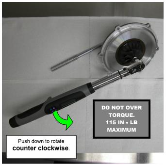
Using an electronic in•lb torque wrench and 6-point, 12mm socket tighten nut securing supercharger impeller to shaft by ROTATING COUNTER CLOCKWISE. NOTE: Threads are left-handed. Torque nut to 115 in•lb by ROTATING COUNTER CLOCKWISE. Threads are left-handed.
