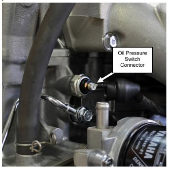
Remove oil pressure switch.
