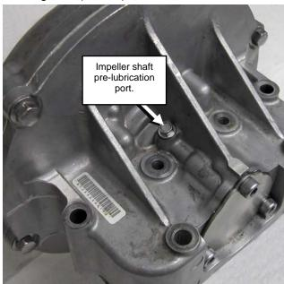
While rotating supercharger impeller slowly add Yamalube 4M engine oil to pre-lubricate impeller shaft.
