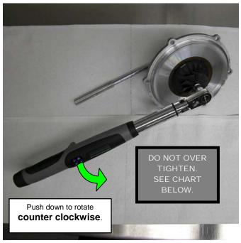
Using an electronic in•lb torque wrench and 6-point, 12mm socket tighten nut securing supercharger impeller to shaft
