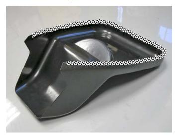
Install air duct back into underside of front storage hatch. Clean up excess silicone. Allow to dry over night before replacing front storage hatch.
