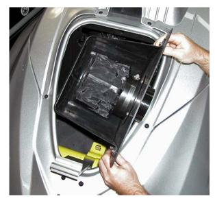
Spray glass cleaner into end of ducting and onto billet flange on back of Power Filter Support. Install end of ducting onto billet flange as shown below. Secure by tightening bolt on billet band clamp. **NOTE: Do not over tighten bolt.**
