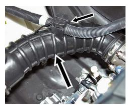
Remove air box lid (8 clips/2 on each side) with filter and discard.
