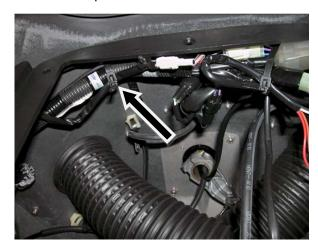
Insert supplied Power Filter Support into front storage compartment.
