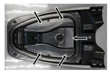
TIP: Use various sized hole saw bits to make initial openings. Fine tune shape with a dremel tool.
