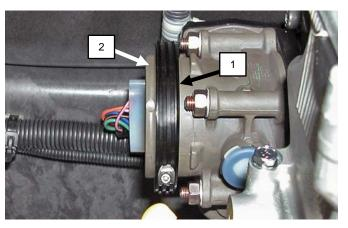
Install supplied tapered plastic flange onto billet adapter flange. **NOTE:** Plastic flange and billet adapter are threaded. Do not over tighten.
