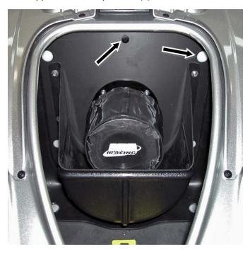
**TIP:** Push center pin of stock rivets out from long end so it is exposed at top of rivet head. Insert rivet and push center pin in so it is flush with rivet head.
