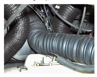
Spray glass cleaner into end of ducting at motor and onto tapered plastic flange on throttle body. Install end of ducting onto flange as shown below. Secure by tightening bolt on billet band clamp. **NOTE: Do not over tighten bolt.**
