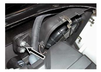
**Optional** – Remove nuts (4) securing air box support bracket to hull. Remove bracket and discard.
