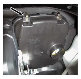
Remove bolts (4 total/2 on each side) securing air box case to support bracket. Remove air box case and discard.
