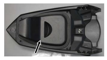
Remove air duct and apply a 3/16" bead of silicone to inside and outside edge.
