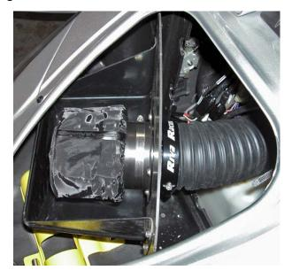
Secure Power Filter Support to hull with stock rivets (5) and supplied rivet at top center (1).
