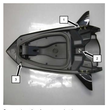
Separate inner liner from storage hatch cover.
