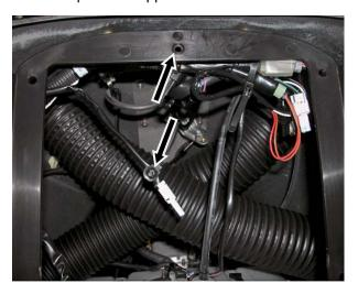
Relocate wire to main wire loom and secure with reusable stock zip tie.
