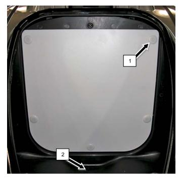
TIP: Push center of rivet in to release.
