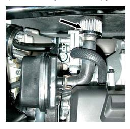
Remove air inlet hose between stock air box and throttle body (2 clamps) and discard. **NOTE:** Cut zip tie securing fuel hose to top of air inlet hose.
