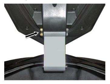
Remove storage hatch from hinge and place on a soft, clean working surface.
