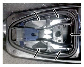
Replace inner liner, hood latch, and mirrors. NOTE: Apply a small dab of silicone to bolts & screws. Do not use Loctite. Do not over tighten.
