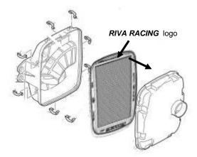
With Performance Air Filter in place on lid, reinstall lid onto air box and secure air box clips (8).
