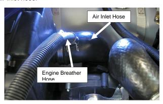
**HO Models:** Disconnect engine breather hose from air inlet hose located between air box & throttle body. Remove air inlet hose.
