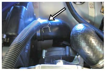
Remove hose between stock air box and supercharger and discard.
