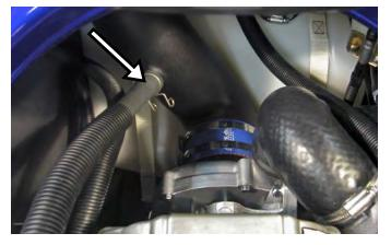
Secure using stock spring clamp.
