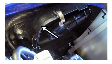
Remove air filter case mounting bracket (4 nuts & washers) and discard. (optional step)
