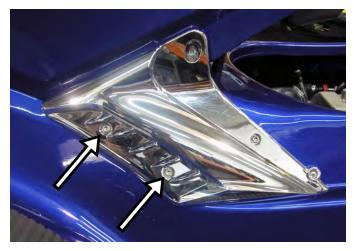
Remove the two socket head cap screws at the leading edge and discard.
