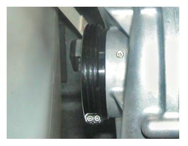
NOTE: The side with the small shoulder must face the supercharger housing. DO NOT USE LOCTITE. Bolts come equipped with thread locking agent. Do not over tighten bolts.
