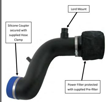
Thoroughly clean both ends of supplied Power Filter tube and inside of supplied Power Filter with a non-residual cleaner. Install supplied Power Filter onto end of tube with threaded brass insert and secure.
