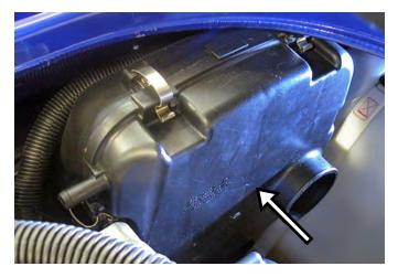
Remove air filter case mounting bolts (4 total -2 on each side) and then air filter case. Discard bolts and case.
