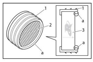
Place rubber holder<sup>1</sup> around outside of supplied billet sleeve<sup>3</sup>. **NOTE: Direction of supplied billet sleeve<sup>3</sup> is critical. Arrow points to side that must face throttle body.**
