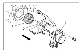
Remove bolts (4) securing joint plate<sup>2</sup> to intake manifold. Remove joint plate and set aside.
