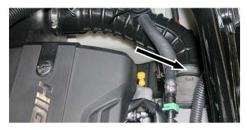
Remove nuts (4) securing throttle body<sup>1</sup> to joint plate<sup>2</sup>.
