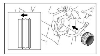
Replace joint plate and secure. **NOTE: Apply blue Loc**tite to bolts. Torque to 17.7 lbf•in / 24 N•m.
