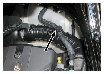
Remove fuel supply hose from mount by lifting up. (Rubber mount is split at top.)
