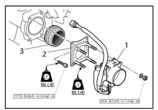
Replace throttle body and secure. **NOTE: Apply blue Loc-tite to studs.** Torque to 9.6 lbf•in / 13 N•m.
