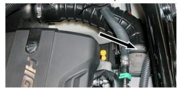
Remove hardware securing throttle body 1 and joint plate 2.
