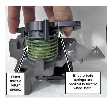
Rotate throttle wheel clock-wise one full rotation, line up opening in center of throttle wheel with throttle shaft and install.
