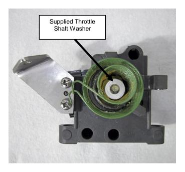
Place supplied throttle wheel onto inner throttle return spring.
