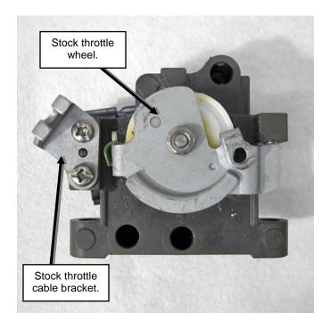
Install supplied throttle cable bracket onto throttle controller assembly and secure with stock Phillips head screws. **NOTE: Use red Loc-tite on threads. Do not over tighten screws.**
