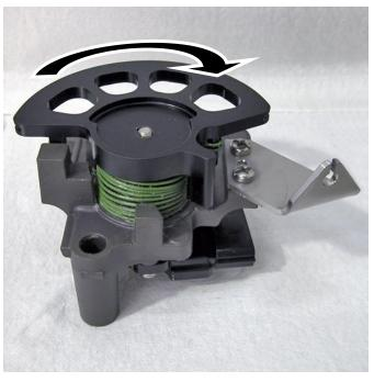
Rotate further to install throttle wheel onto throttle shaft completely. Install stock lock washer and throttle shaft nut onto throttle shaft and tighten. (see illustration below)
