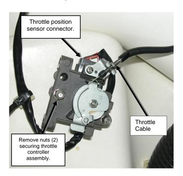
Remove stock throttle wheel with plastic spring retainer and throttle cable bracket from throttle controller assembly and discard. Retain Phillips head screws, nut & washer. NOTE: Do not pry throttle wheel with any tools. Pull upward applying even pressure. Use care when removing as springs will uncoil rapidly.
