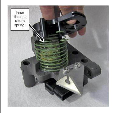
Place throttle wheel into outer throttle return spring. (see illustration below)
