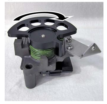
Rotate further to install throttle wheel onto throttle shaft completely. Install stock lock washer and throttle shaft nut onto throttle shaft and tighten. (see illustration #10)
