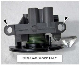
Replace throttle controller assembly in hull.
