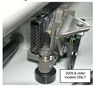
Reconnect throttle position sensor connector. **NOTE: Make sure connector "snaps" into place.**
