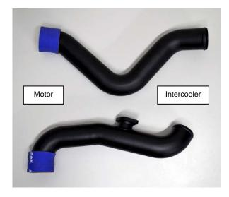
Install intercooler to throttle body tube. Secure with supplied clamps and stock clamps. **NOTE: Do not over tighten clamps.**
