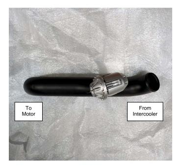
Install supercharger to intercooler tube. Secure with supplied clamps and stock clamps. **NOTE: Do not over tighten clamps.**
