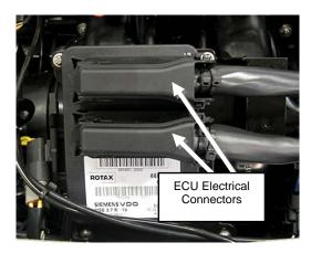
Remove bolts (4) securing ECU to ECU mounting plate. Remove ECU and set aside.
