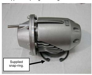
Place blow-off valve on top of billet flange so vacuum tube is facing throttle body. While pressing down on valve secure snap-ring into groove using 45-degree snap-ring pliers.
