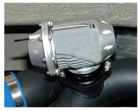
NOTE: Ensure snap-ring securely locks into groove in billet mounting flange.
