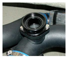
Install supplied o-ring into o-ring groove in billet mounting flange.
