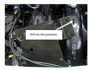
Using the supplied 3/32" drill bit carefully and slowly drill straight into the end of the protrusion. **NOTE: The** material you are drilling into is made of thin plastic. Do not push or force drill bit. Drill slowly.
