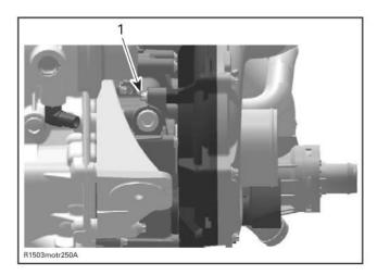
Remove supercharger unit from engine.
