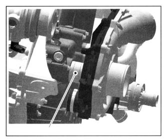
Install supercharger unit onto engine. **NOTE**: It may be necessary to rotate supercharger impeller to allow supercharger gear to mesh with flywheel gear.
