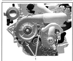
Remove supercharger unit from engine.
