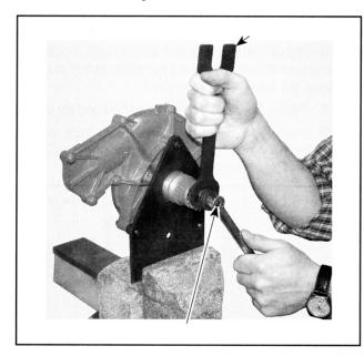
Remove nut, angular ring and spring washer pack. Discard spring washers.
