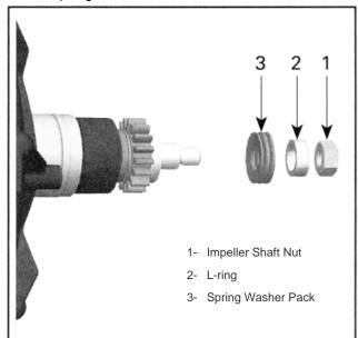
Carefully clean exposed portion of supercharger impeller shaft with a non-residual cleaner.
