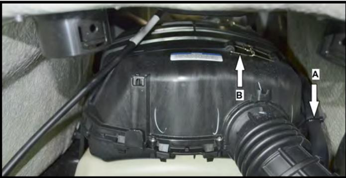
Release clamp (A) holding OEM inlet tube to airbox hose. Cut zip tie (B) securing wire harness to OEM inlet tube. (Figure 9)
