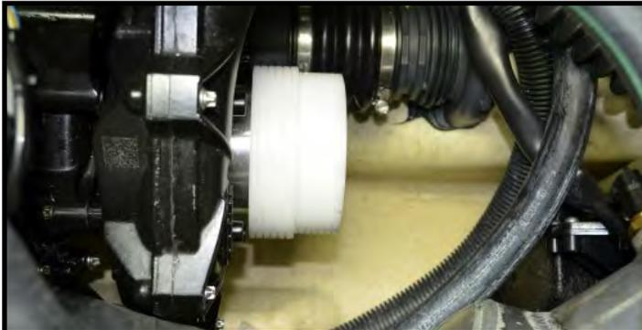
Slip supplied 2" silicone coupler onto velocity stack. Slide two supplied hose clamps loosely over silicone coupler. Tighten clamp closest to engine only. (Figure 15) **Tip: Spray glass cleaner on inside of coupler and outside of Velocity Stack to ease installation.**
