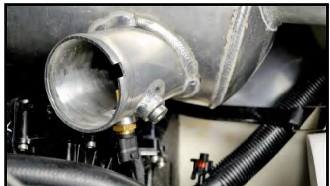
Reinstall waterbox and coupler assembly onto exhaust manifold reversing removal procedure. **NOTE: Do not tighten hose clamp yet. Tip: Lubricate inside of coupler and outside of exhaust manifold with glass cleaner to ease installation.**
