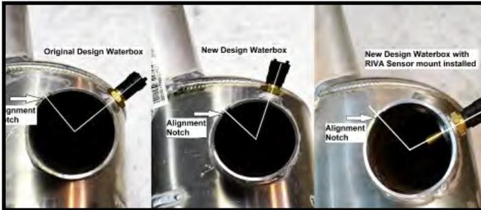
Note that the location of the temperature sensor is changed in relation to the index notch on the waterbox outlet. The new location of the temperature sensor interferes with Inlet Tube A of this kit. **If your ski is equipped with one of these waterboxes the sensor must be re-located to install this kit.**
