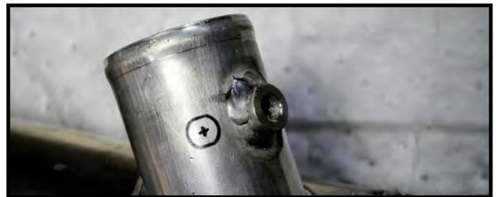
Hole center should be at 3:00 to 4:00 position with respect to index notch in waterbox tube. (see figure EX1)
