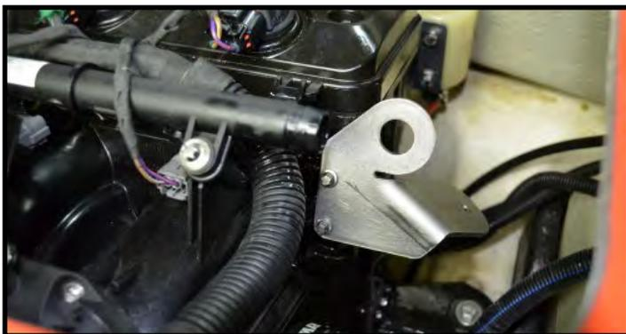
Loosen bolts in supplied threaded ring and slip over supercharger inlet. Note: Assemble ring so that both ring halves have two dots showing. (This will align threads in both halves.) Position threaded ring against flare on su-
