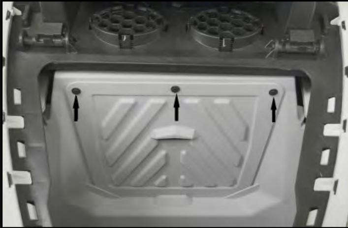
Pull out on the tabs to release the vent tubes and pull vent tubes down and out of the hull. (Figure 2)
