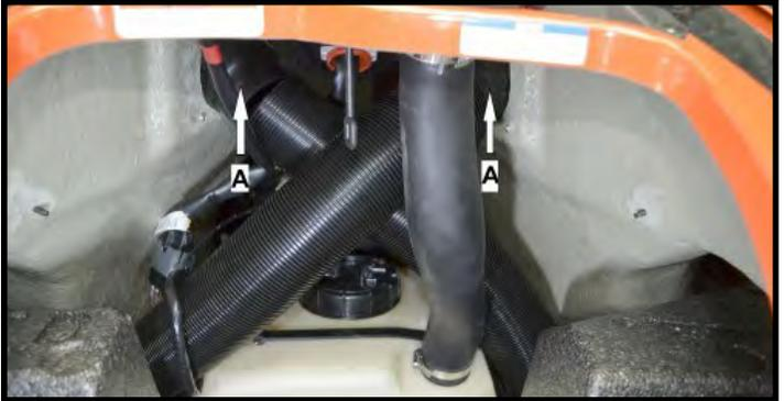
Loosen clamp (A) and remove fuel filler hose from tank.
